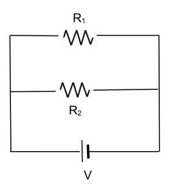
We consider two resistors  $R_1$  and  $R_2$  in parallel, as shown. The potential drops across the two resistors  $V_1$  and  $V_2$  is equal to the voltage of the battery:  $V = V_1 = V_2$ . Since  $I_1 = V/R_1$  and  $I_2 = V/R_2$  are the currents through the resistors  $R_1$  and  $R_2$ , respectively, the current through the battery is the sum  $I = I_1 + I_2$ . We introduce the equivalent resistance  $I = V/R_{eq}$  and find
